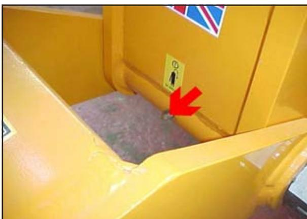
Fig. 5.18: Drawbar Pivot Grease Point
