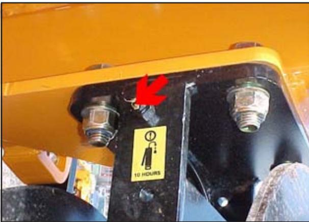
Fig. 5.08: DD Roll Grease Points
