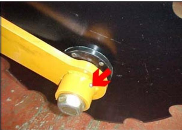
Fig. 5.10: Coulter Coverer Grease Points
