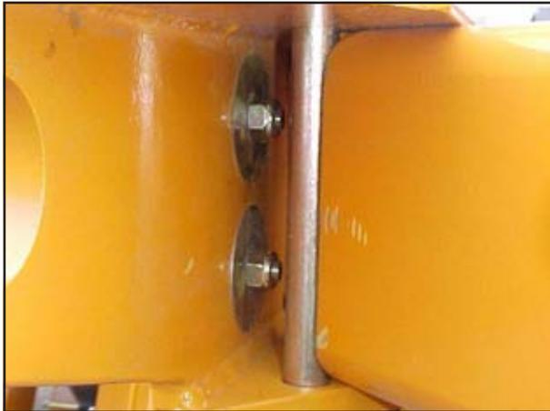
Fig. 5.01: Inner Tine Beam Shims
