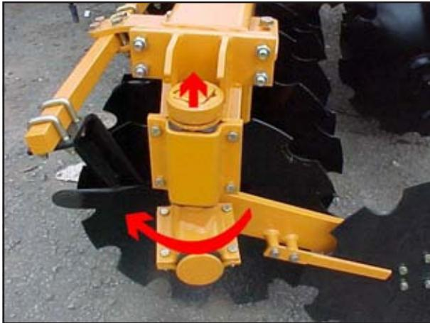
*Fig. 4.04: RH Coulter Coverer (shown in transport position).*
