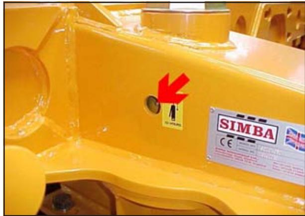
Fig. 5.11: Gang Pivot Grease Points
