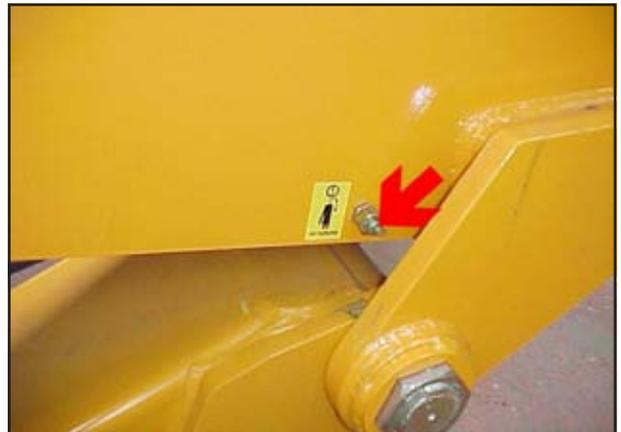
Fig. 5.15: Transport Axle Pivot Grease Point
