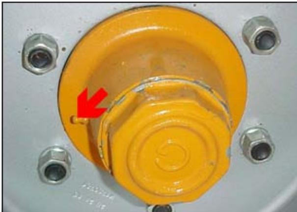
Fig. 5.14: Wheel Hub Grease Points
