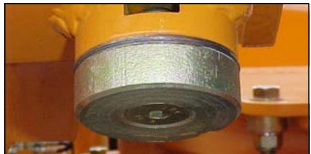
Fig. 5.04: Roll Wing Shims
