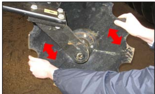
Fig. 5.01: Checking Disc Bearing Adjustment
