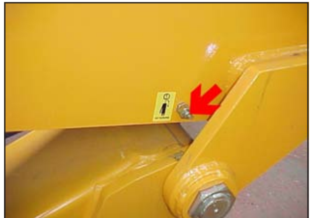
Fig. 5.15: Transport Axle Pivot Grease Point
