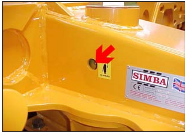
Fig. 5.11: Gang Pivot Grease Points
