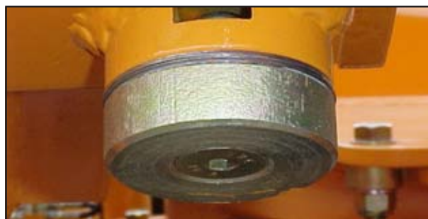
Fig. 5.04: Roll Wing Shims
