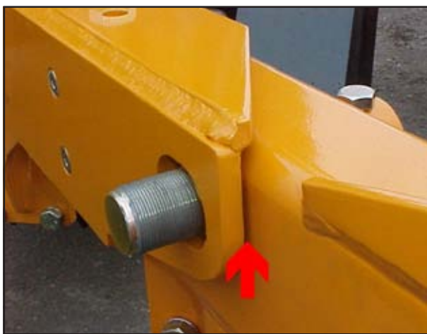
Fig. 5.02: Tightening the Tine Beam
