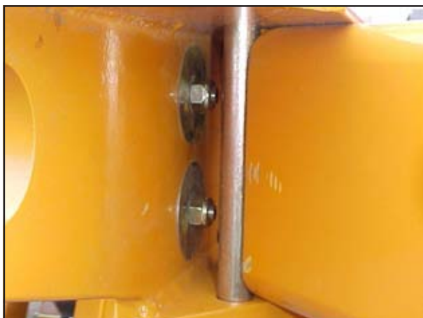
Fig. 5.01: Inner Tine Beam Shims
