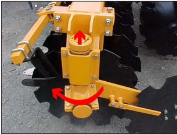
Fig. 4.04: RH Coulter Coverer (shown in transport position).
