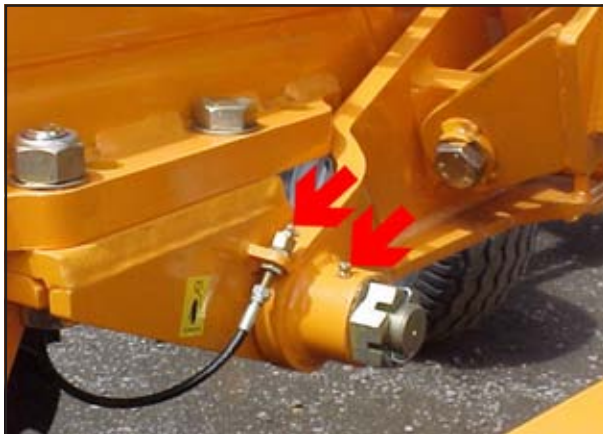
Fig. 5.16: Roll Carriage Pivot Grease Points
