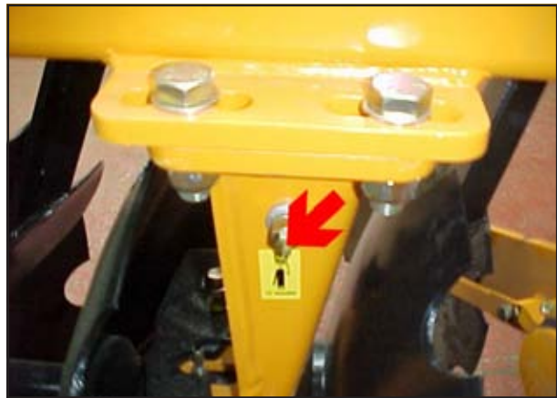
Fig. 5.09: Disc Axle Grease Points
