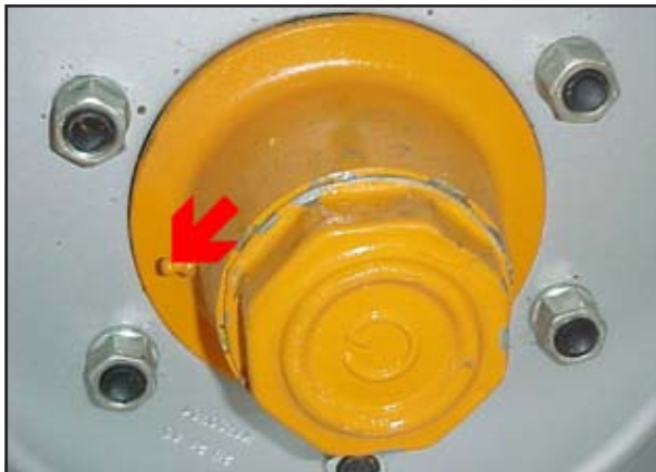
Fig. 5.14: Wheel Hub Grease Points
