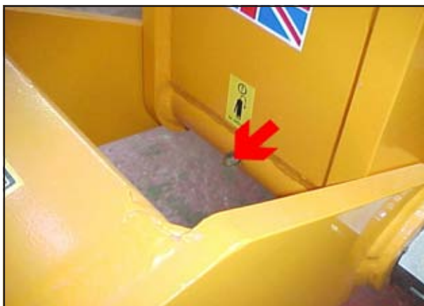
Fig. 5.18: Drawbar Pivot Grease Point
