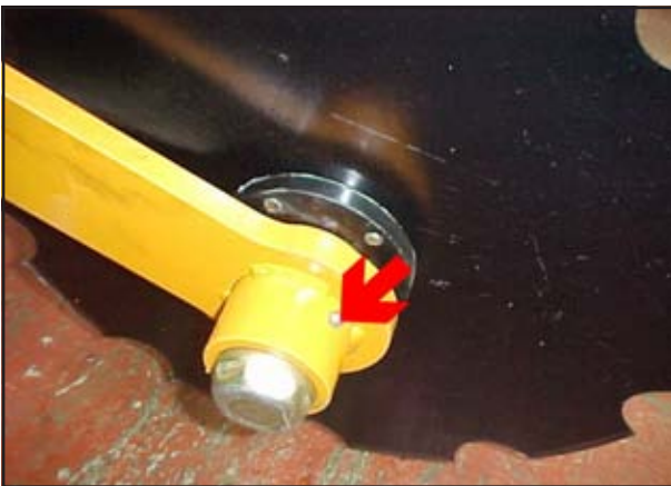
Fig. 5.10: Coulter Coverer Grease Points
