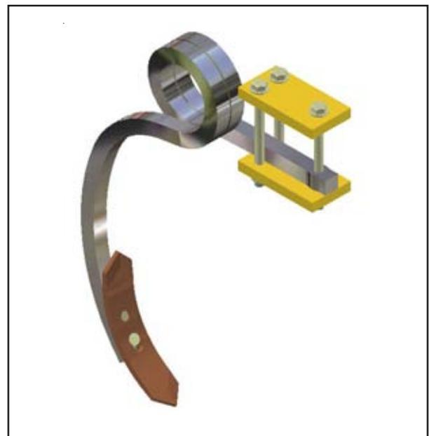
Fig. 3.05: Horizontal Pigtail Tine
