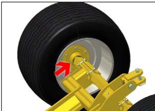
Fig. 5.10: Wheel Bearing Grease Points
