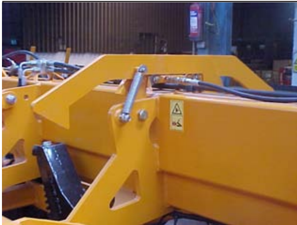
Fig. 2.02: Automatic Wing Lock
