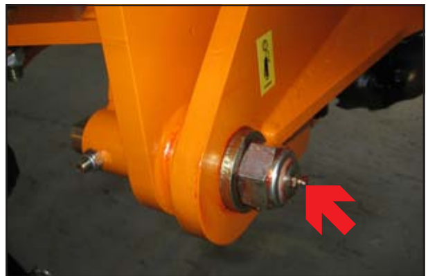
Fig. 5.09: Wing Pivot Grease Points
