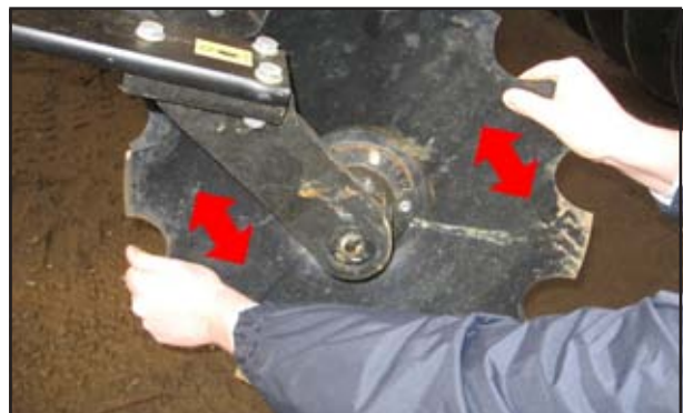
Fig. 5.01: Checking Disc Bearing Adjustment
