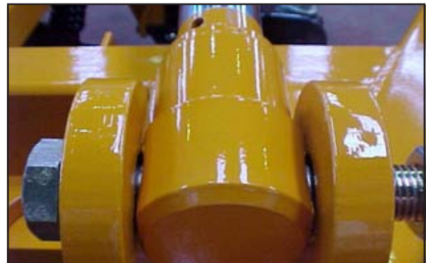
Fig. 5.04: Wing Pitch Adjustment - Solo 450
