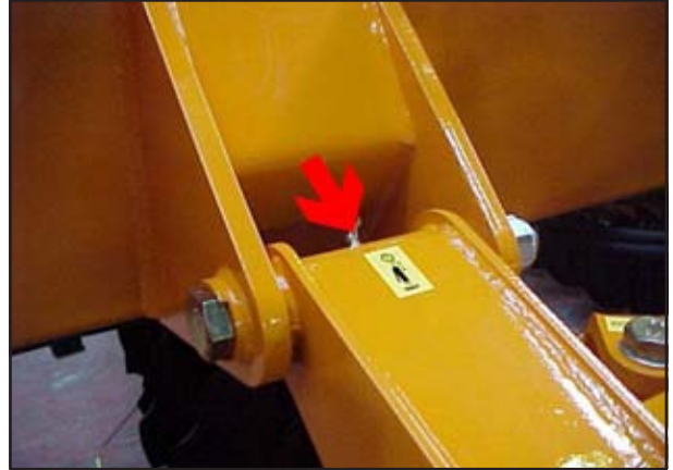
Fig. 5.13: Wing Pivot Grease Points
