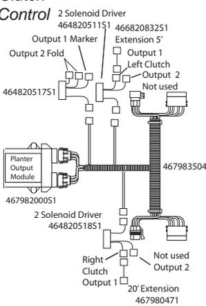
Note: Connect the WSMT Actuator harness and the Dj Planter Harness to the mating connectors of the WSMT Module harness
