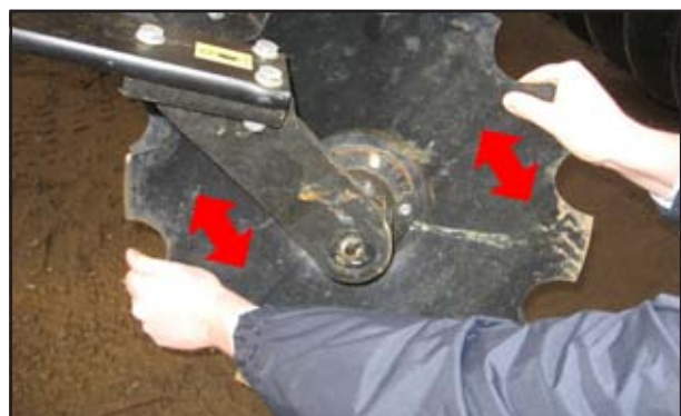
Fig. 5.01: Checking Disc Bearing Adjustment
