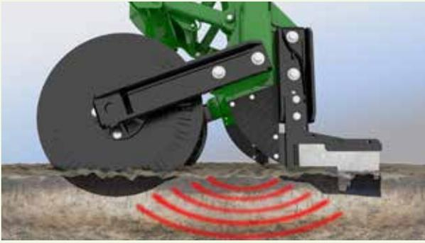
Electrical conductivity is one of the ways to identify soil types, as each type conducts electricity differently. TrueView uses electrical currents that pass between the sensor and the coulters to measure these variations in soil type and texture.
